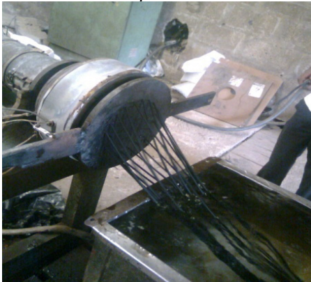
Figure 1: Polyethylene rod coming out of the machine
