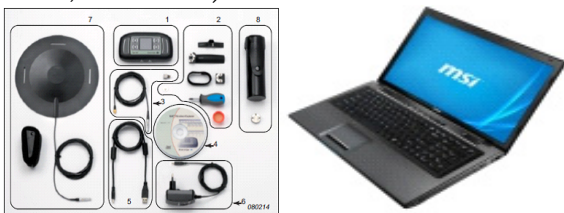
Figure 5. Equipment that was made measurement: type 4447 analyzer and computer processing of measurements in 4447 Vibration Explorer-software. The main accent in the measurement is the position of the Z axis, set as vertical and horizontal component when measuring.
