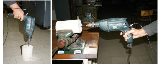
Figure 8. Machine B- Small Hand Drill ( \Phi 5 ) Working with Small Hand Drill Machine in vertical and horizontal positions
