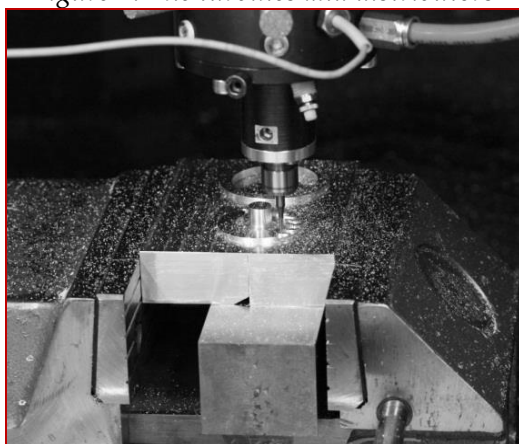
Figure 5: Production of radial air turbine and distributor
