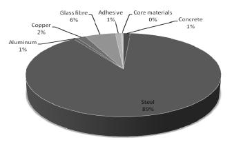
*Figure 2 – Distribution of raw materials in wind turbines without foundations (1.5 MW) [17]*
