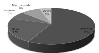
Figure 3 – Material distribution in a 40 meters and 7 tons rotor blade [16]
