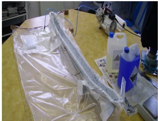
Figure 7: Vacuum pressed technology
