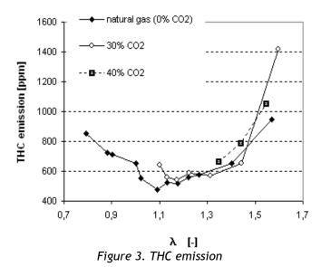
In Figure 3 it can be discovered that considering the incombustible hydrocarbon content of the exhausted gases there is no significant deviation present between the operation of natural gas and gas mixtures with a higher carbon-dioxide content in the range of  $\lambda$ =1.2-1.4 air access ratio.
