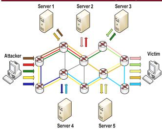
Figure 2. Principle of Reflective Denial of Service
