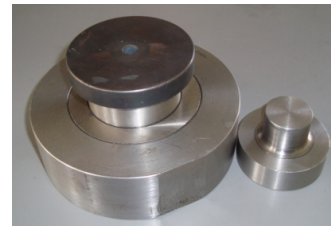
Fig. 8 - Compressing tool for die
