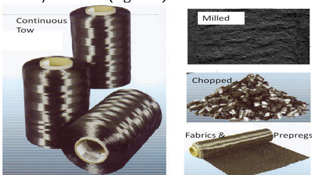
Figure 8. Product forms of carbon fibers
