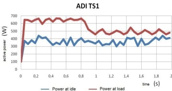
Figure 9. Comparison of power active components at idle and at load in drilling one hole
