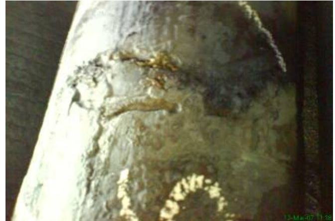
Fig. 11. Interruption in the physical continuity of the casting
