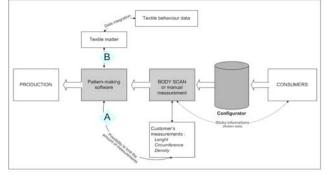
Fig. 1. Configuration for Clothing Mass Customization
