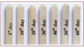
Fig. 9 Specimens biodegradation in NEUTRAL area
