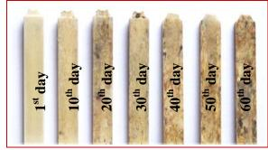
Fig. 11 Specimens biodegradation in NATURE COMPOST
