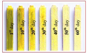
Fig. 8 Specimens biodegradation in ACIDIC/ALCALIC area – graphically exposed
