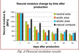
Same reason of flexural modulus change caused relatively high decrease of flexural strength as shown on fig. 3.
