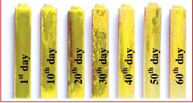
Fig. 10 Specimens biodegradation in NEUTRAL area - graphically exposed
