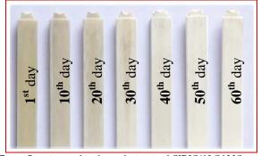
Fig. 7 Specimens biodegradation in ACIDIC/ALCALIC area.
