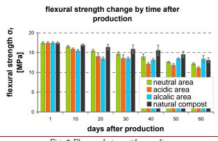
Fig. 3 Flexural strength results
