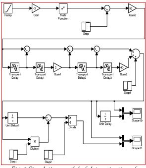
Fig. 1 Simulation model of determination of predictive limit temperature.
