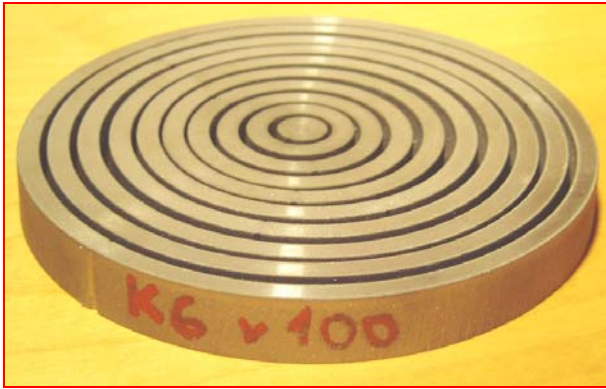
Fig. 5. An example of rings cut in steel plate
