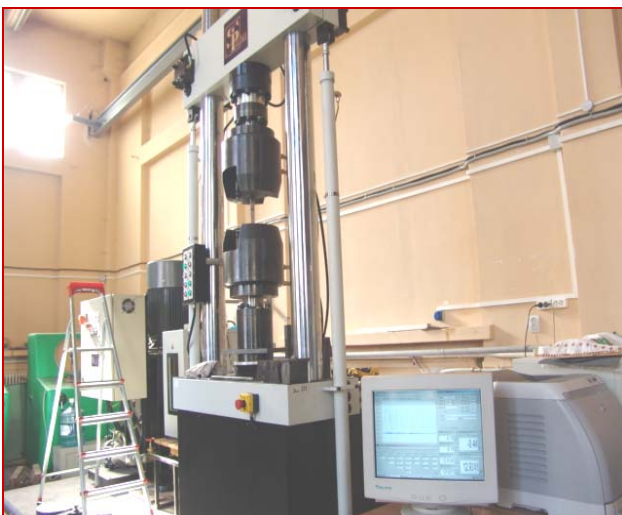
Figure 1 The Universal Testing Machine SI-PLAN 942-1 type
