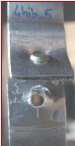
Figure 5. Adhesive break Figure 6. Metal break
